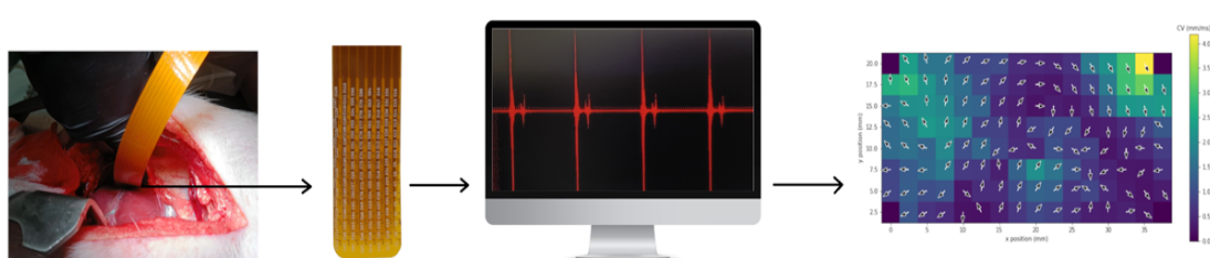
Figure 2: MEA setup. From left to right: in an open-chest state, the MEA was placed on the left atrial epicardium. The MEA was able to simultaneously record 64 unipolar electrograms. From differences in local activation times, conduction velocity maps were derived. MEA = multi-electrode array
